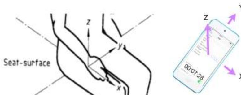
*Fig.9 Burgess-Limerick 2014 iOS Application User Manual shows the positioning under the drivers ischial tuberosity on left or right.*
